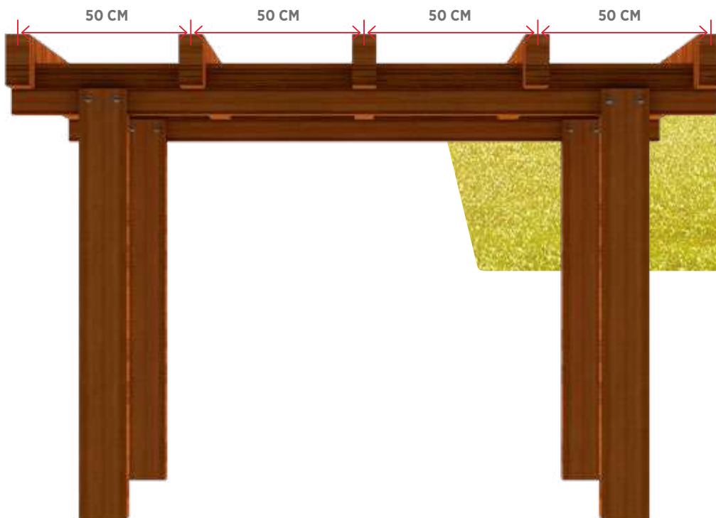
1 – Measure the rafter
